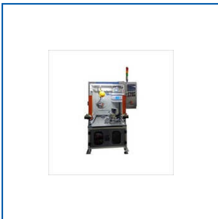
LEAK TESTING MACHINE FOR TCL CONNECTION
